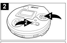
press the MODE/◀ button ❷ repeatedly until the mode indicator disappears.
