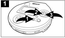
To repeat all files in a directory (MP3 CD only), while in the Stop mode, press the MODE/◀ button ● three times; "REP D" will appear in the display. Press the Skip/TUNING DN |◀◀ ❷ or UP ►> ❸ button to select the specific directory that you wish to repeat.
