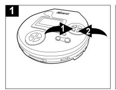
During playback, depress and hold either the Skip/TUNING DN |◀◀ ● or UP ▶▶ ● ● button to move the player forward or backward within a track to locate a specific musical passage. The player will move forward or backward at high speed as long as the buttons are depressed. When you release the Skip/TUNING DN |◀◀ ● or UP ▶▶ ● ● button, normal playback will resume.
